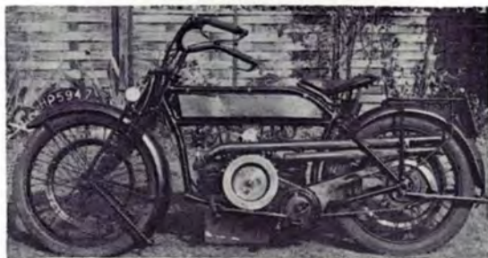
Above: A 1923 Humber 600 c.c. horizontally-opposed twin cylinder model. This machine has belt-rim brakes back and front.
