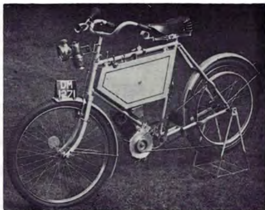
Above: A 1923 Humber 600 c.c. horizontally-opposed twin cylinder model. This machine has belt-rim brakes back and front.
